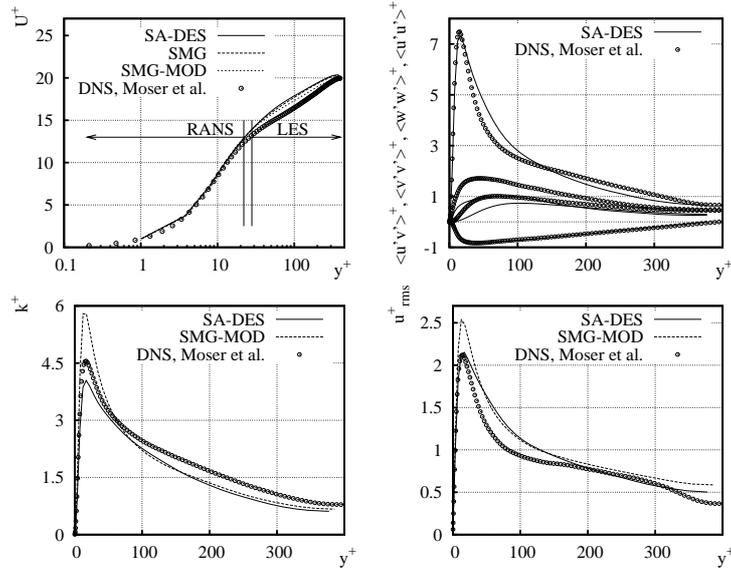
**Fig. 3** Channel flow  $Re_\tau = 395$  for modified Smagorinsky and SA-DES model: Upper left: Mean velocity  $U^+$ . Upper right: Fluctuations. Bottom left: Kinetic energy  $k^+$ . Bottom right:  $u_{rms}^+$ .
