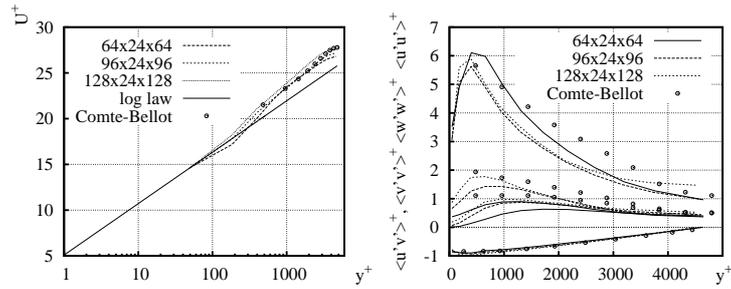
**Fig. 4** SA-DES model with near-wall modeling (WSADES) for channel flow  $Re_\tau = 4800$ .
