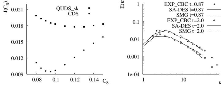
**Fig. 1** Left: Calibration of Smagorinsky constant  $C_S$  for DIT. Right: Energy spectrum with optimized model constants of Smagorinsky model and of SA-DES model for CDS scheme.
