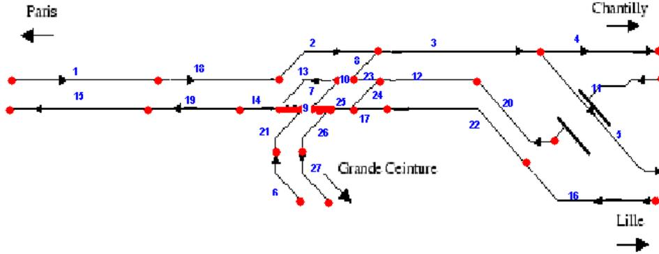
Figure 2: Layout of the junction Pierrefitte-Gonesse subdivided into track sections.
