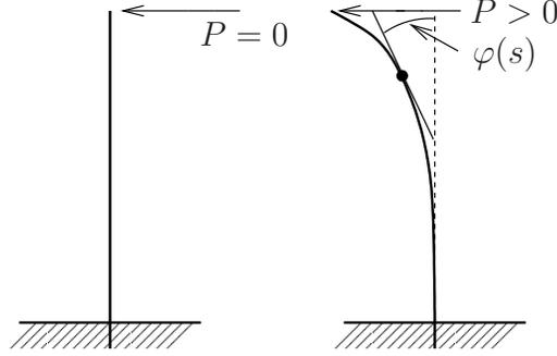
Figure 1: Rod with load perpendicular to the rod
