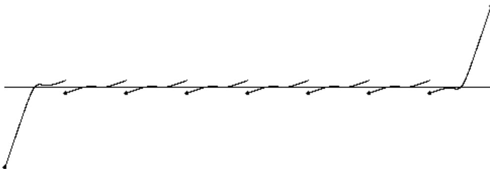
**Figure 8.** Derivative of curvature of  $S3$  interpolant of order 6.
