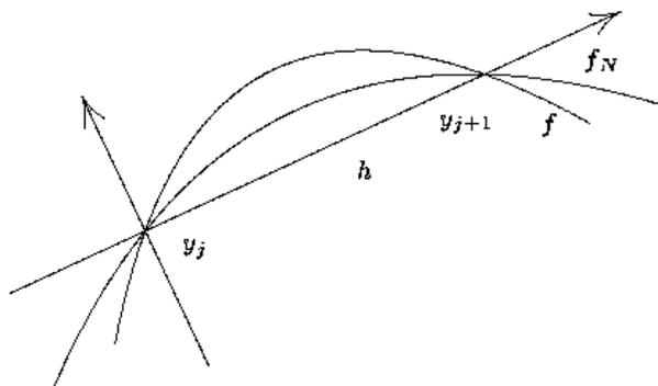
**Figure 1.** Error between curve and interpolant.
