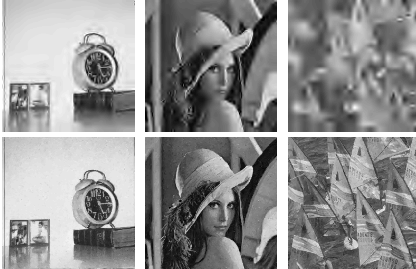
Fig. 1: Top row: Reconstruction by tensor-product wavelet compression using the 7-9 biorthogonal filter bank with 1000 wavelet coefficients for test image clock (PSNR 29.93), 700 coeffs for Lenna (PSNR 24.28), and 200 coeffs for sail (PSNR 19.58). Bottom row: Reconstruction by EPWT wavelet transform using the 7-9 biorthogonal filter bank with 1000 wavelet coefficients for clock (PSNR 33.55), 700 coeffs for Lenna (PSNR 30.46), 200 coeffs for sail (PSNR 27.19).
