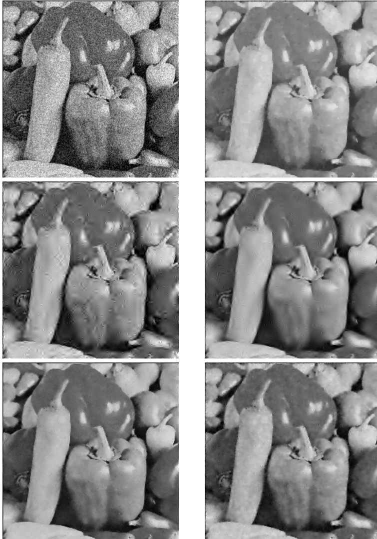
Fig. 2: Top row: Peppers with additive white Gaussian noise with \sigma = 25 (PSNR 19.97) and reconstruction by the Four-Pixel Scheme [29] (PSNR 28.26), Mid row: Reconstruction by 2d tensor product wavelet transform using the 7-9 biorthogonal filter bank without (PSNR 24.91) and with cycle spinning (PSNR 28.11) Bottom row: Reconstruction by our approach described in Subsection 2.3 using a relaxed path construction with fixed local distances in (2), (PSNR 29.01) and a random path construction based on (4) (PSNR 27.96).
