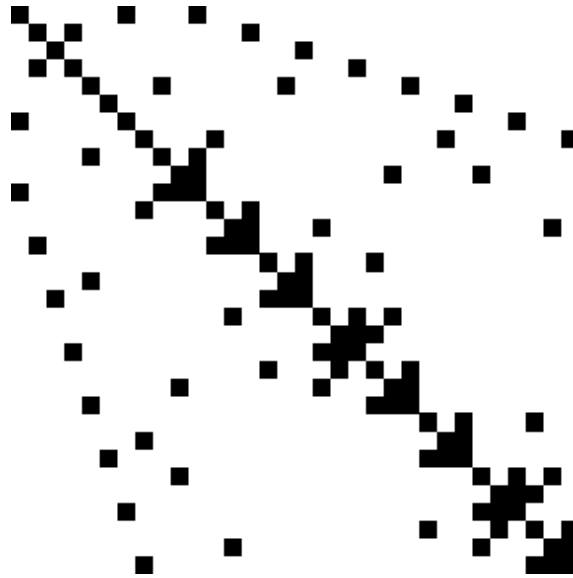
Figure 1.5.2: Sparsity Pattern of DG for the problem 1.4.3 and the initial mesh (see also Figure 1.4.1(b)) for polynomial degree p = 10 (Matrix has the size 2112 \times 2112 ).
