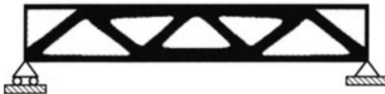
Figure 1.1: Optimized truss structure (image taken from [BS13, p. 2]).
